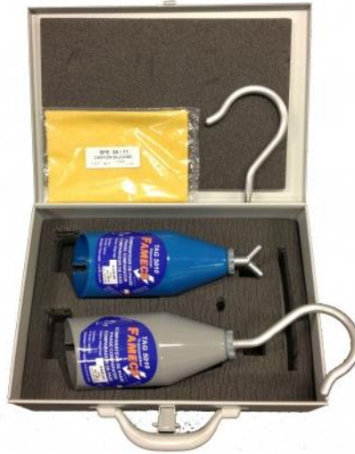
Figure 10-9 HV overhead wireless phasing out equipment
