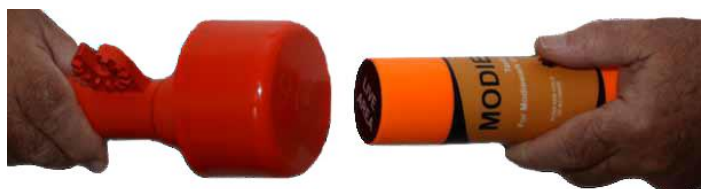
Figure 10-3 The Modielive® EMF generator (right) used to test the integrity of the Modiewark's testing function.
