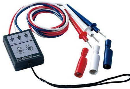
Figure 10-16 Typical phase rotation meter
