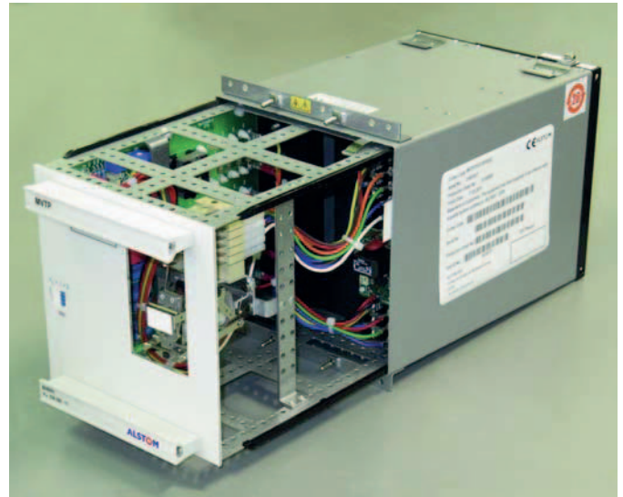
Figure 7.4: Busbar supervision static relay
