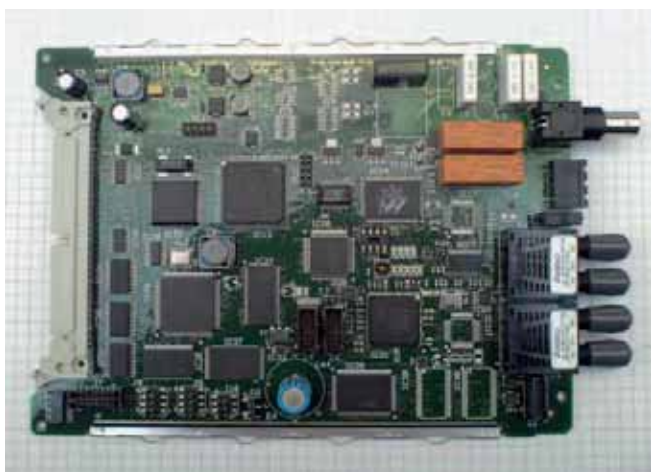
Figure 7.10: Numerical relay redundant Ethernet board
