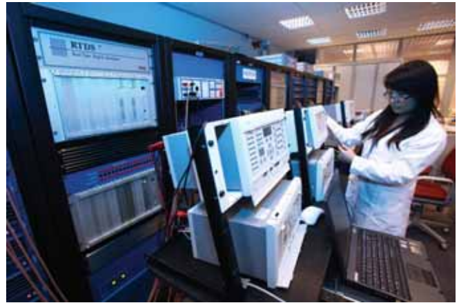
Dynamic simulator scheme approval for a numerical IED
