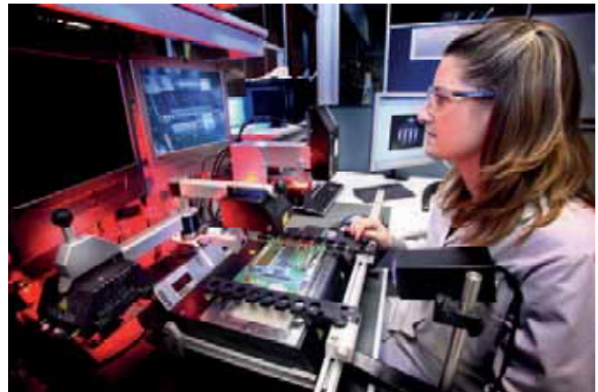
Figure 7.16: Quality inspection of a numerical relay printed circuit board
