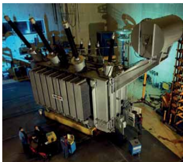
Figure 5.11: Testing a high voltage transformer
