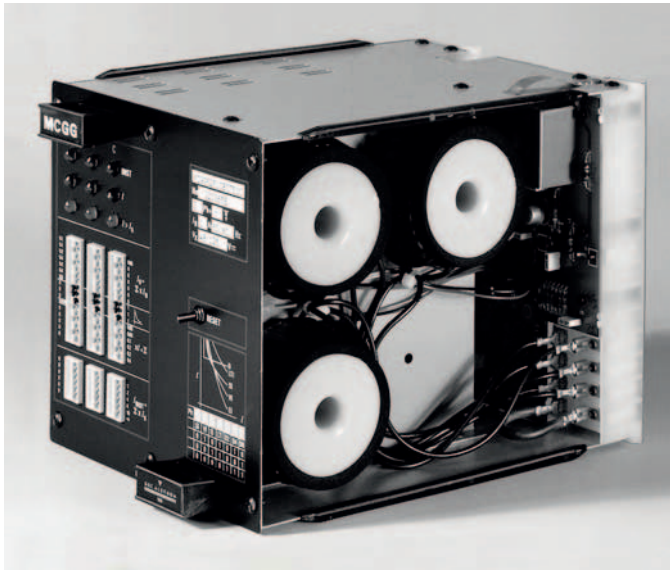
Figure 7.5: Second generation distribution digital relay (1982)
