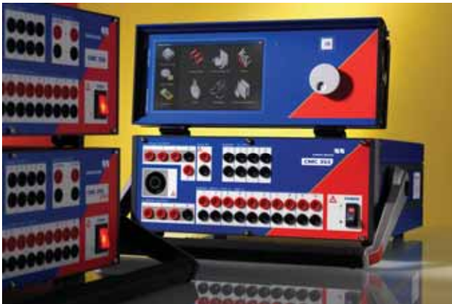
Figure 21.21: Modern PC-based secondary injection test set
