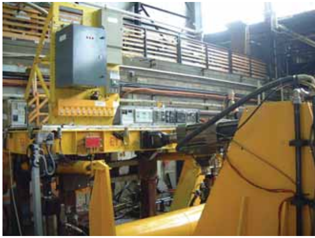
Figure 21.10: Relay undergoing seismic test
