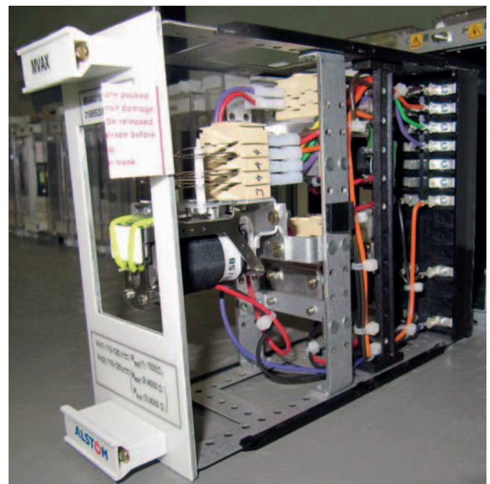
Figure 7.3: Attracted armature relay in manufacture
