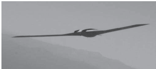
Wing-span - 28 metres; AUM - 4090 Kg Powerplant – Two, 13.4 KN thrust Williams FJ44 Turbo-fans Predicted Operational Altitude - 30,000 metres (~100,000 ft)
