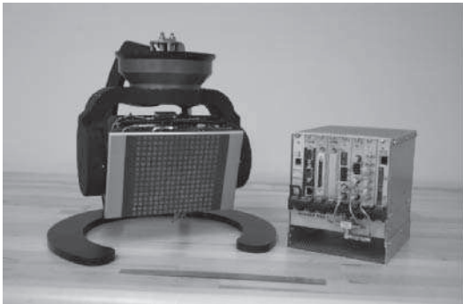
Figure 8.7 Lynx synthetic aperture radar systems
