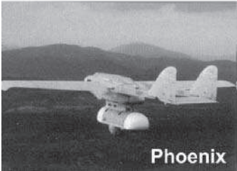
Figure 4.17 Close-range UAV systems: Observer and Phoenix (Reproduced by permission of Cranfield Aerospace Ltd)
