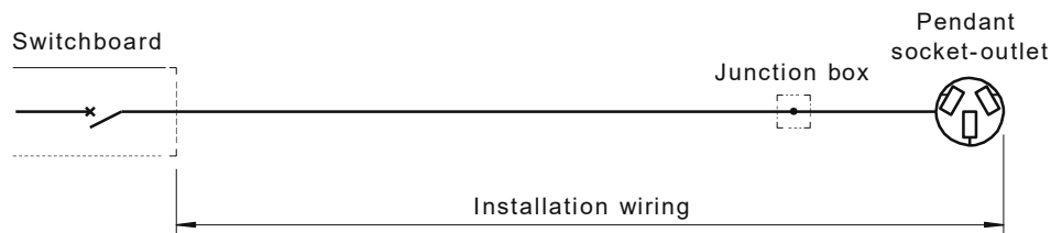
FIGURE 4.8 EQUIPMENT WIRING—EXCEPTION FOR PENDANT SOCKET-OUTLET
