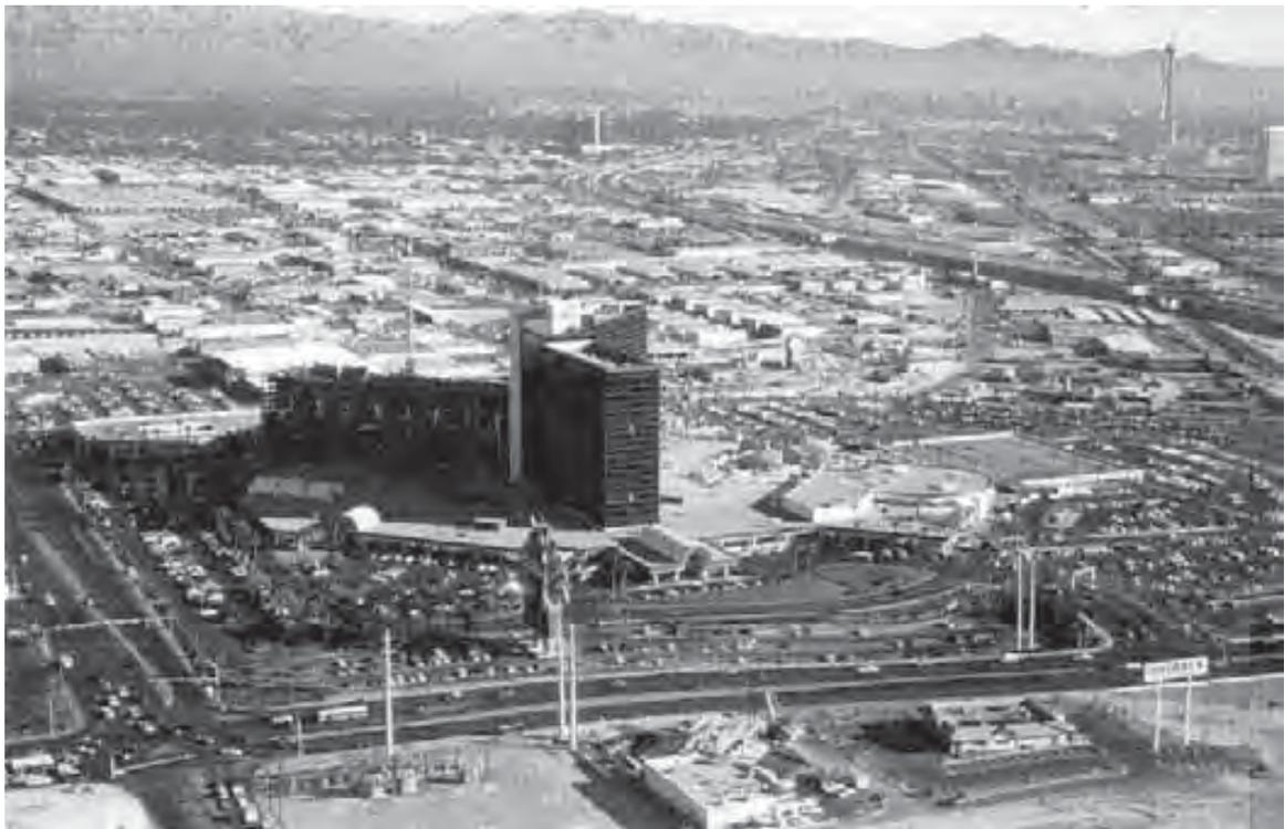
**Figure 1.13d.** Structure in the foreground is located in exposure B. Structures in the rear, adjacent to the clearing, are located in exposure C when wind flows from the left over the clearing.
