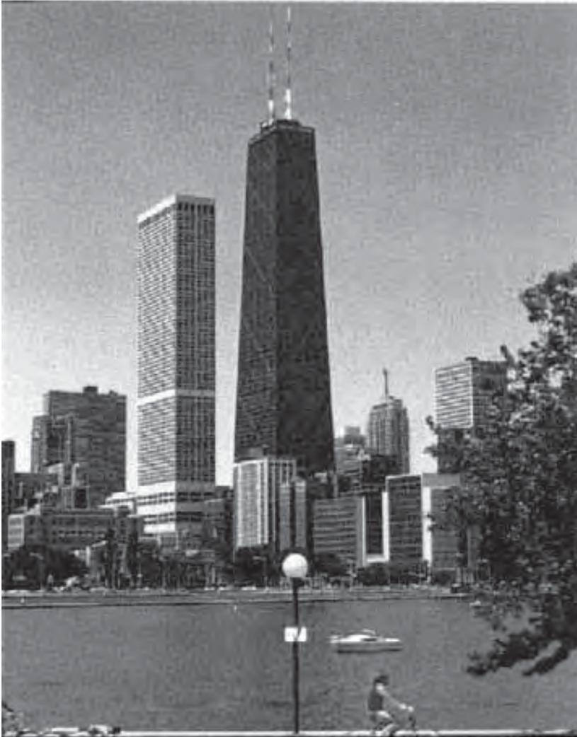
**Figure 1.13e.** Structures on a shoreline with wind flowing over open water for a distance of at least one mile are located in exposure D.
