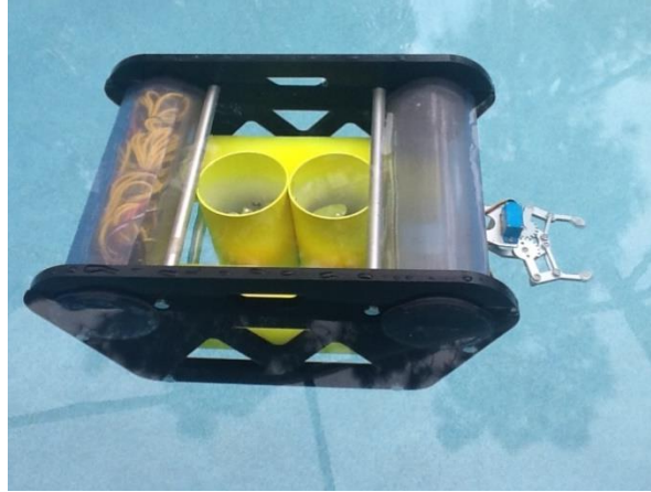
Figure 17: ROV in near full assembly in water
