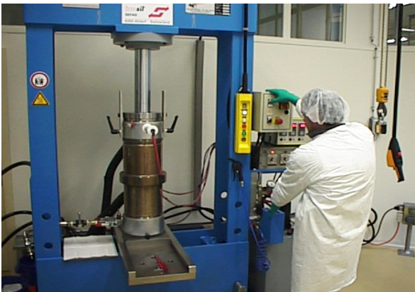
Picture 10: View of a production station for insulating material in clean room environment
