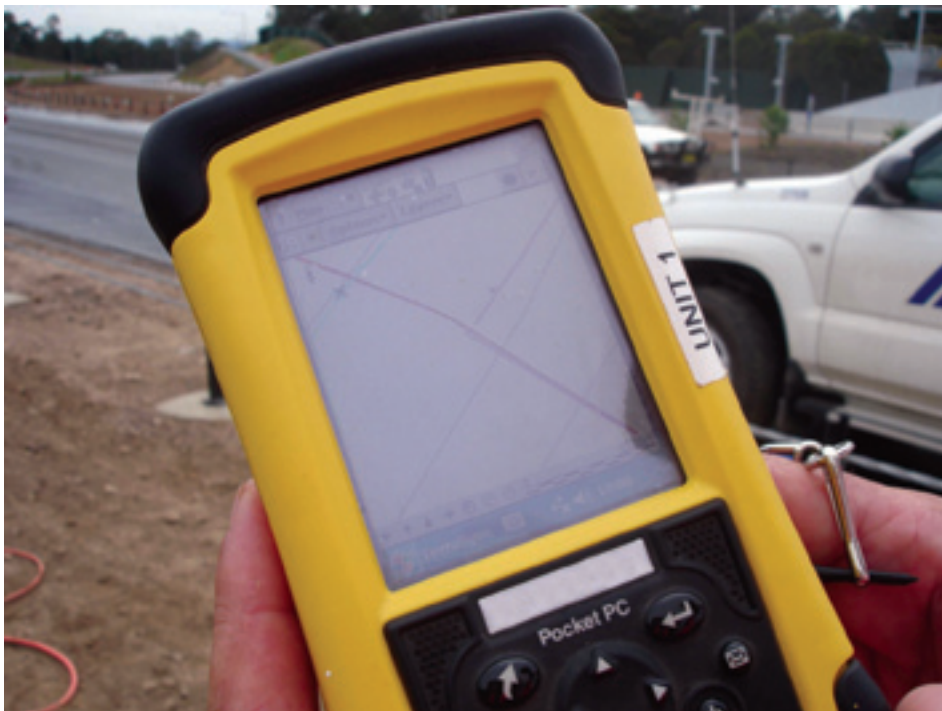
The manufacturer's pocket PC allows quick recognition of underground assets by touch screen technology. This identifies the type of asset and its approximate location.
