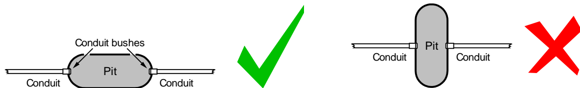
Figure 5 Right and wrong use of intermediate pits
