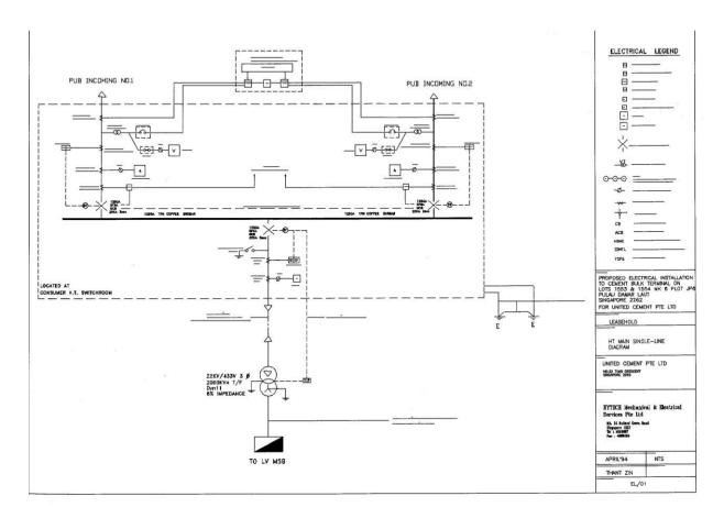
The above diagram is Incoming HV supply system for a Cement Factory. It contains Star –Delta Transformer, Interchange switches for switching 2 supply, sketch of protective relay system with trip circuit and outline for measuring instruments.
