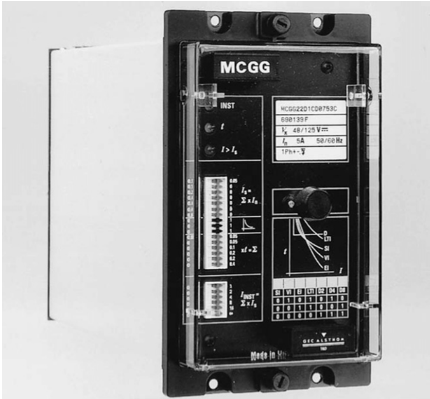
Figure 10.7d Modern microprocessor controlled solid state IDMTL relay – type MCGG. A wide variety of characteristics is available. PSM and TSM settings are configured using the small switches accessible from the front of the relay (courtesy GEC Alstom T & D Protection & Controls)
