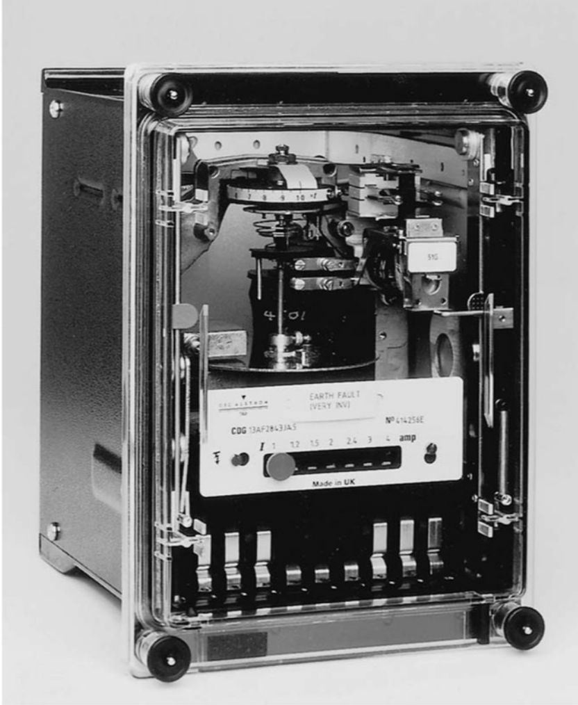
Figure 10.7b Traditional electromechanical IDMTL relay. The illustration shows an earth fault relay (type CDG) with a 'very inverse' characteristic. The plug settings are at the front of the relay and time settings at the top (courtesy GEC Alsthom T & D Protection & Controls)
