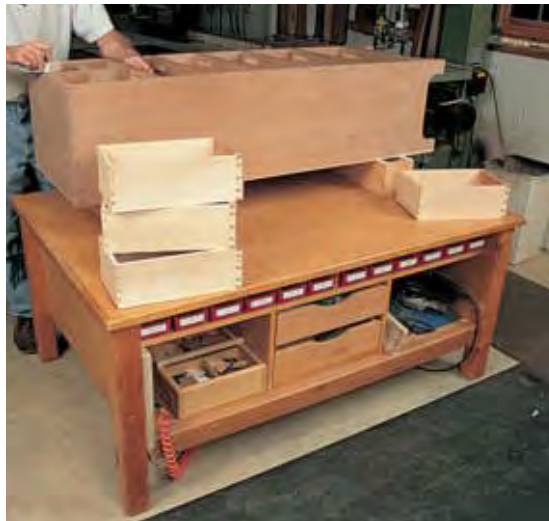
A low work table for assembly, clamping, and sanding will help save your back.
