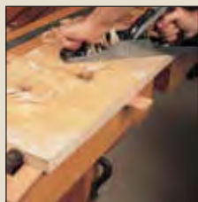
27 Flattening a Board by Hand
