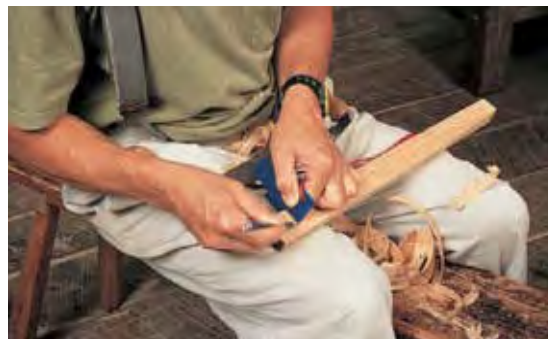
Once two adjacent faces are worked square, Langsner uses a simple shop-made gauge to mark out the width of the piece.
