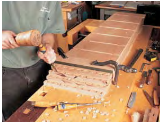
A holdfast uses a wedging action through the benchtop to keep a piece in position for handwork, especially for carving or chopping tasks.
