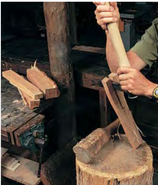
Used as a lever, the froe quickly separates individual squares from the blank.
