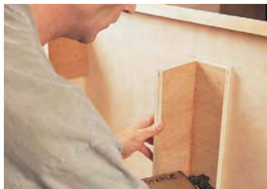
Staples and glue secure the foot to the underside of the cabinet.
