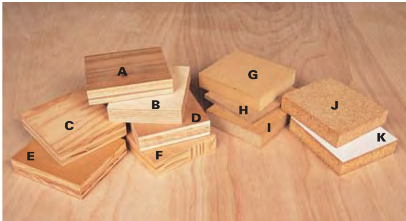
A , Hardwood veneer-core plywood with walnut face; B , Baltic birch plywood, C , softwood plywood with fir face; D , combination-core plywood with cherry face; E , MDO; F , lumbercore with birch face; G , MDF; H , hardboard (for example, Masonite); I , solid core of MDF with oak face; J , particleboard; K , MCP.
