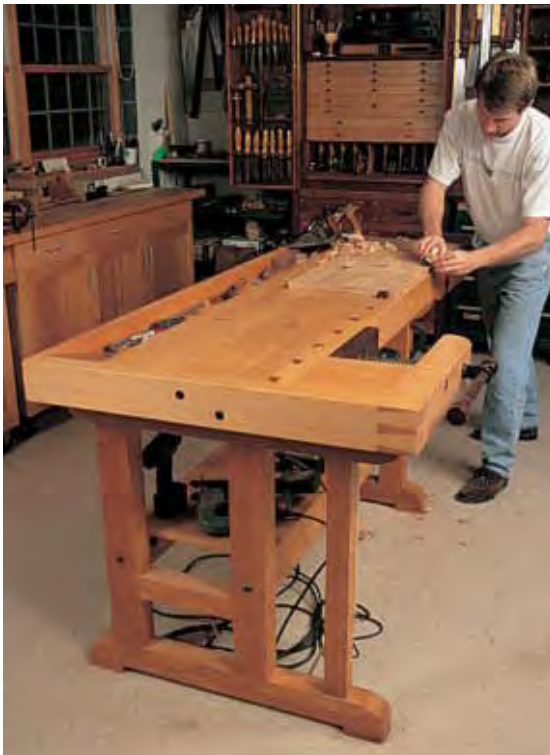
Pinching the workpiece between bench dogs helps pull it flat to the benchtop, especially useful when handplaning.
