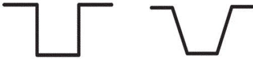
Fig. 6.30 Channel cross-sectional design for advanced high-strength steel with larger included angles to facilitate manufacturing. Source: 6.3
