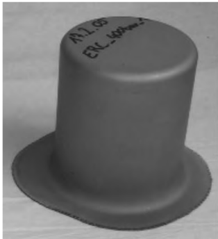
Fig. 8.23 Results of research study in sheet hydroforming with punch. (a) Pot pressure curve and optimum blank holder force (BHF) curve predicted using numerical optimization techniques coupled with finite-element modeling. (b) Wrinkles in the round cup were eliminated by using optimum BHF.
