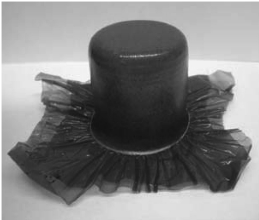
Fig. 5.21 Polytetrafluoroethylene film used in warm forming. Source: Ref 5.14
