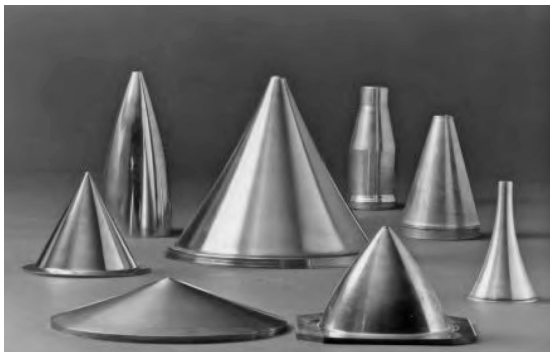
Fig. 12.40 Example parts manufactured by shear spinning. Source: Ref 12.15
