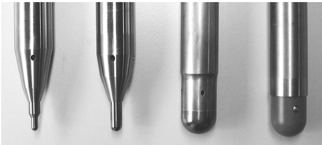
Fig. 13.6 Forming tools (left to right): satellite tools with radii of 3, 5, and 15 mm, respectively, and a 15 mm plastic tool. Source: Ref 13.3
