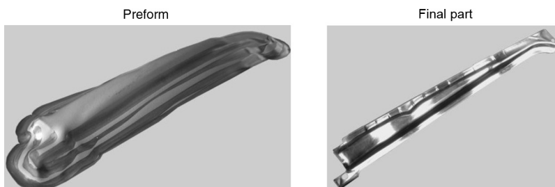
Fig. 13.17 Stiffening brace manufactured by incremental sheet metal forming. Source: Ref 13.9
