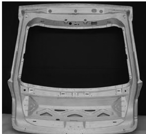
Fig. 5.39 Chevrolet Malibu Maxx lift gate manufactured by using quick plastic forming. Source: Ref 5.35
