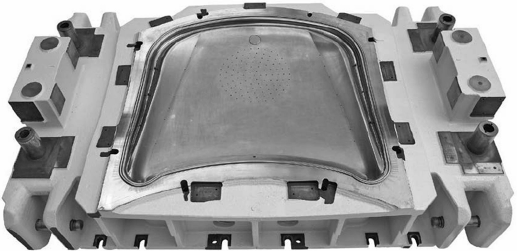
Fig. 16.11 Ion-nitrided forming tool for hood outer panel. Source: Ref 16.48
