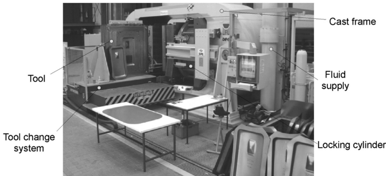
Fig. 8.11 Schematic of horizontal sheet hydroforming with die press located at the University of Dortmund's Light Forming Technology Center. Source: Ref 8.16
