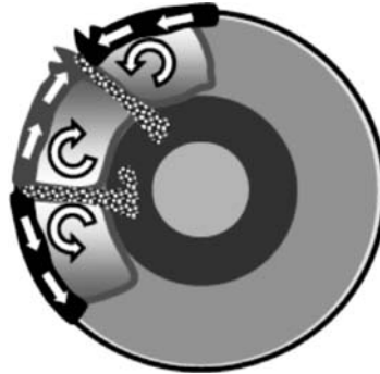
Figure 1.2 Local convective currents in the mantle (Source: Murty, C.V.R. "IITK-BMPTC Earthquake Tips." Public domain, National Information Centre of Earthquake Engineering . 2005. http://nicee.org/EQTips.php - accessed April 16, 2009.)
