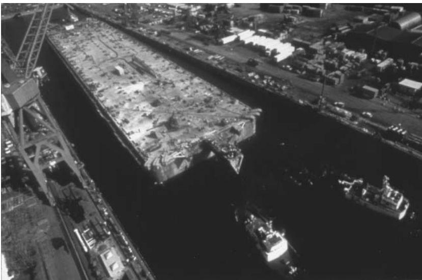
FIGURE 13.11 N'Kossa barge being towed out of dry dock. (Courtesy of Buoygues Offshore.)
