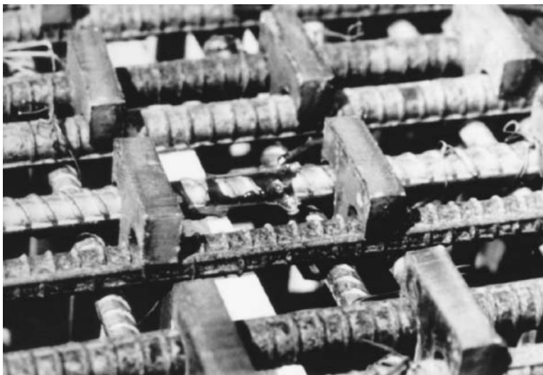
FIGURE 4.11 Headed reinforcing bars.
