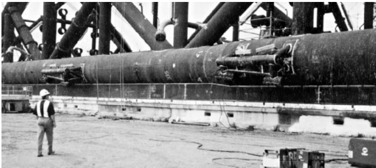
FIGURE 22.8 Connectors at hinge in rigid tubulars in order to allow upper section to be compliant under storm waves. (Courtesy of J. Ray McDermott S.A).
