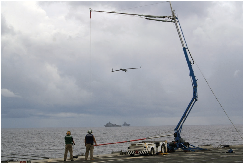
Operators on board a ship prepare to recover a ScanEagle drone Credit: Royal Navy
