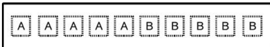
Fig. 2.13 House painting example: naive experimental design, showing a wall (large rectangle) with several test surfaces which are painted using paints A or B.
