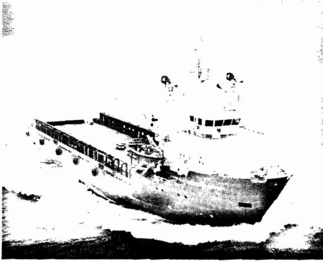
Figure 6.16: The supply vessel Northern Clipper . Length L = 76.2 (m) and mass m = 4.591 \cdot 10^6 (kg).
