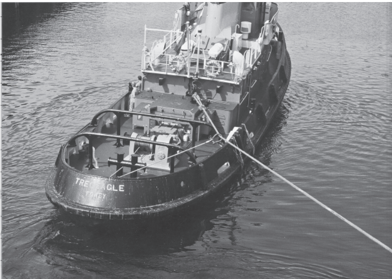
32. Alternative type of gob rope (wire) and electric winch.
