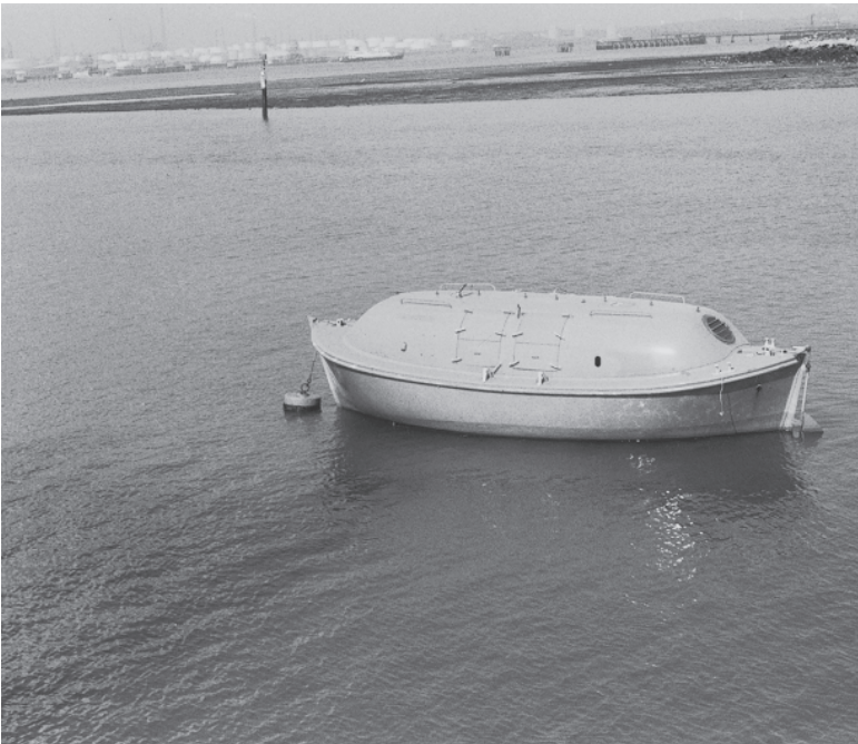
28. Totally enclosed lifeboat on moorings.
