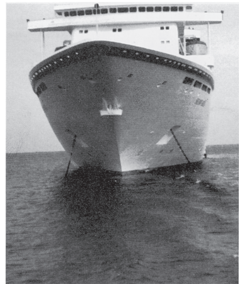
30. Cruise ship moored, deploying both Port and Starboard anchors. N.B. Additional centre anchor in stowed position.
