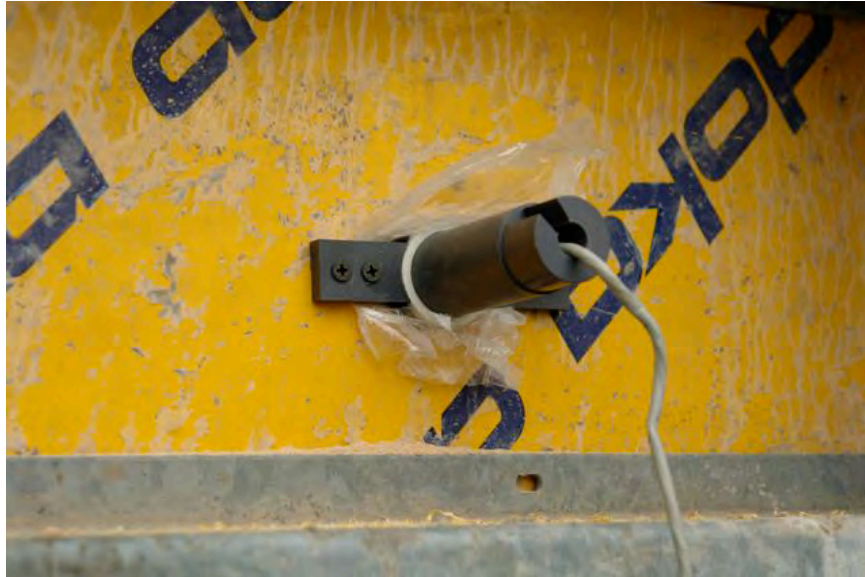
Figure 3 —Bracket with Pressure Transducer Attached to Formwork
