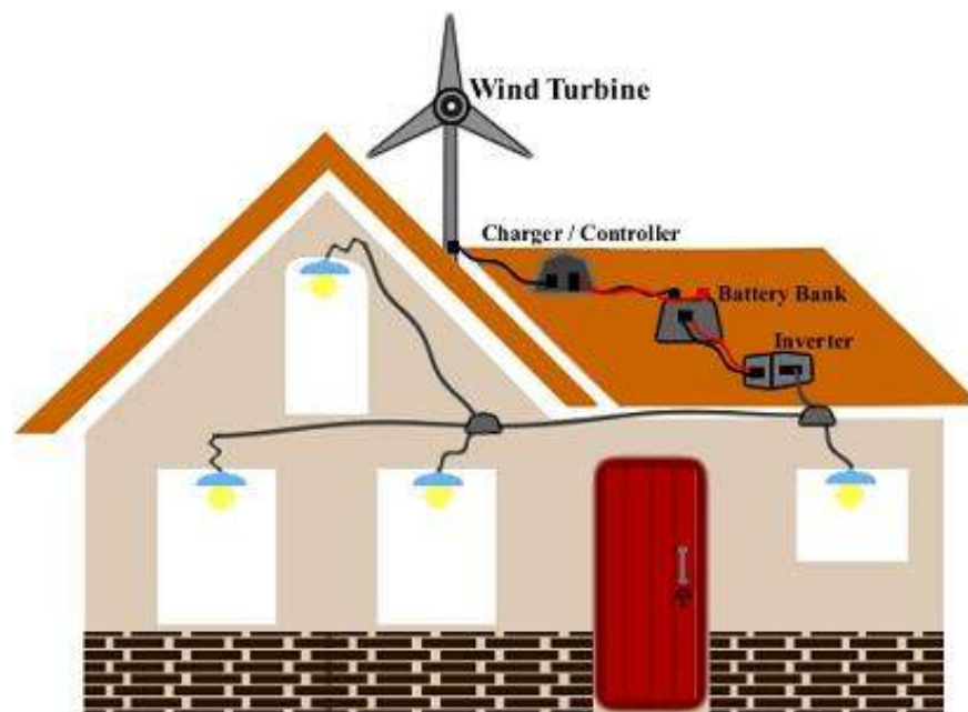
Figure 4.3 Wind Energy System
