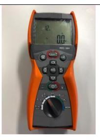
A loop impedance meter is used to provide the impedance of an active and neutral circuit back to the supplying transformer. The incoming service neutral must be disconnected from the installation earthing conductors to prevent a parallel return path through the earth resulting in an incorrect loop impedance reading.
