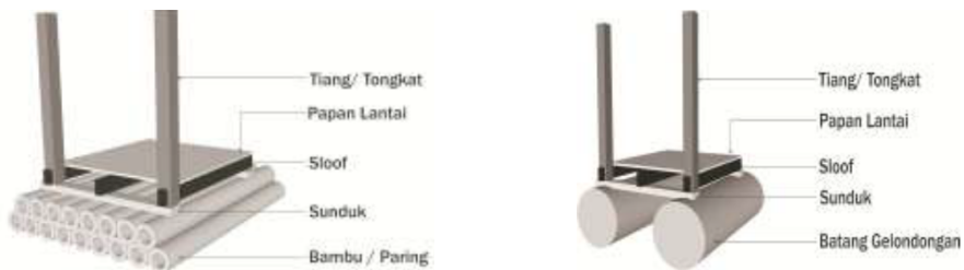
Fig. 7. The Technology of the Structure of Floating Foundation of Lanting house Source: Rahman, 2014
