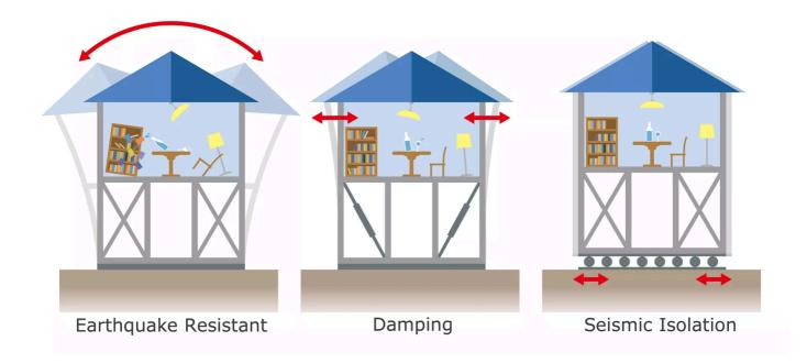
Japan uses many smart ways to build earthquake-safe structures. These methods include both stiff and bendy designs. Each type has its own perks for keeping people safe during quakes.
