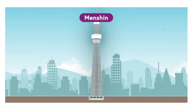
The menshin system, or base isolation, is a key Earthquake Resistant strategy. It uses laminated rubber bearings and dampers. These allow buildings to move horizontally during seismic activity.
