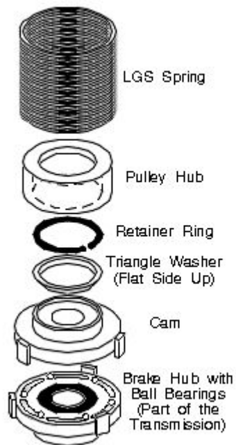
Figure FA-8: GE Washing Machine Lower Bearing
