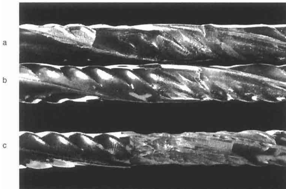
Fig. 19-2 Appearance of the active test pieces in a 6-month experiment according to Fig. 19-1 and Table 19-1. (a) U_{\text{Cu-CuSO}_4} = -0.80 to -0.95 V, (b) U_{\text{Cu-CuSO}_4} = -0.75 to -0.80 V, (c) without cathodic protection, in electrical contact with passive steel.
