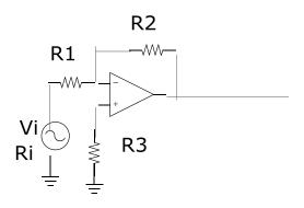
$R1 = 4.7 \text{ K}\Omega$ ,  $R2 = 100 \text{ K}\Omega$ ,  $R3 = 3.3 \text{ K}\Omega$
