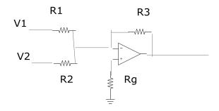
R1= 10 K  $\Omega$  , R2= 4.7 K  $\Omega$  , R3 =100 K  $\Omega$  , Rg = 3.3 K  $\Omega$
