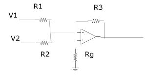
R1= 10 K $\Omega$ , R2= 4.7 K $\Omega$ , R3 =100 K $\Omega$ , Rg = 3.3 K $\Omega$
