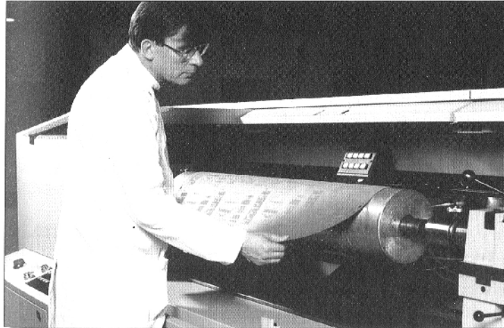
Figure: Operator examining a laser-engraved rubber plate.
