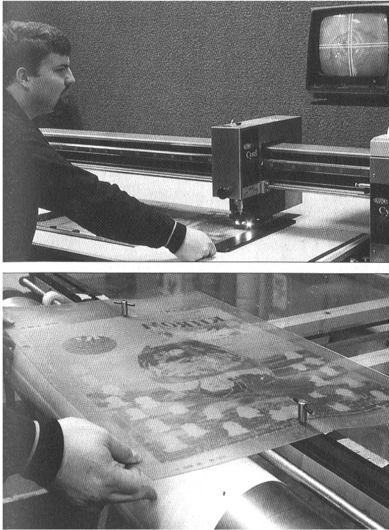
Figure 3.16 - The pin-registration concept. The plate is drilled (top), then pinned to the cylinder (bottom)
