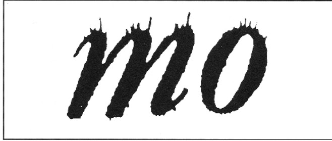
Fig. Gravure print problem - Whiskers (magnified about 15-20x).
