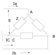
Z = 50 (Angle 0 )  $\Omega$   $\,$  E = 400V. The currents in A,B, C lines are
