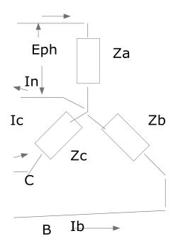
Eph= 100V, Za=  $100\Omega$ , Zb = $100\Omega$  in series with  $66.3\mu$ F, Zc= $100\Omega$  in series with 139.2mH f= 50HZ. Calculate the current in neutral wire (In)
