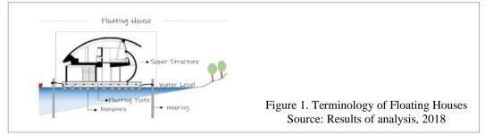
The floating house is above the water with the position of the building following the water level. It needs the principle of balance so that the building is not tilted, and needs a fastening pole so that the house does not move following the flow of water.
