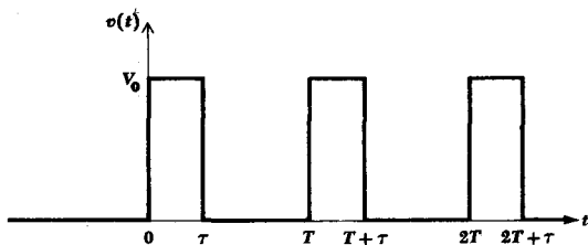
Fig. 19-5 A periodic train of rectangular pulses for which F(s) = (V_0/s)(1 - e^{-s\tau})/(1 - e^{-sT}) .
