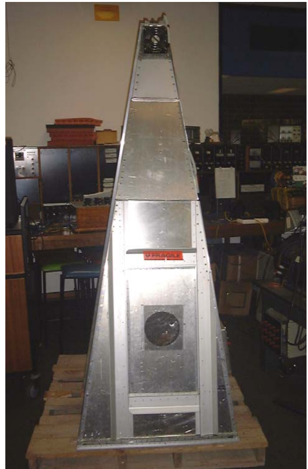
Figure 5: The completed G-TEM cell.
