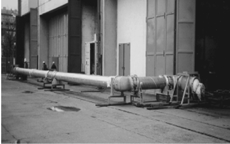
FIGURE 18.11 High-current and internal-arc test setup. (Courtesy of Siemens.)
