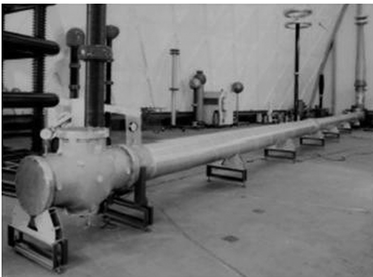
FIGURE 18.13 Test setup for high-voltage tests. (Courtesy of Siemens.)
