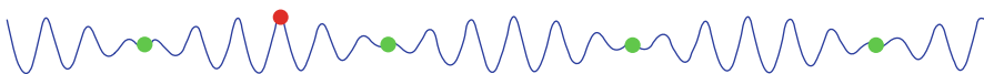
Fig. G.9 Frequency dispersion in groups of gravity waves on the surface of deep water [3]
