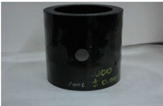
Fig. 1.3 Fiber composite compression cylinder with 1.0-in.-diameter pin
