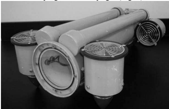
Fig. 3 Robot chassis and thrusters with floatation units
