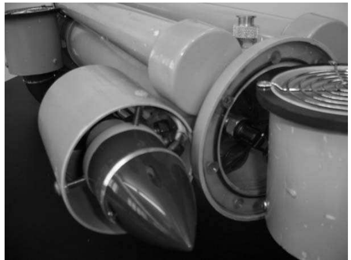
Fig. 5 Thruster showing bilge pump
