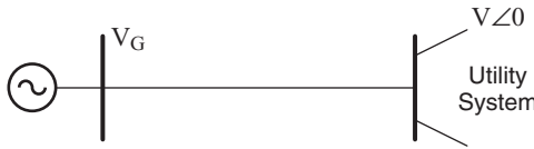
Figure 2.30 A Generator Operating with a Lagging Power Factor.
