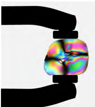
Figure 27.49 Optical stress analysis of a plastic lens placed between crossed polarizers. (credit: Infopro, Wikimedia Commons)
