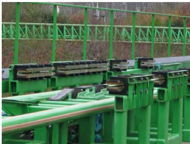
Figure 23.19 The rows of rare earth magnets (protruding horizontally) are used for magnetic braking in roller coasters. (credit: Stefan Scheer, Wikimedia Commons)
