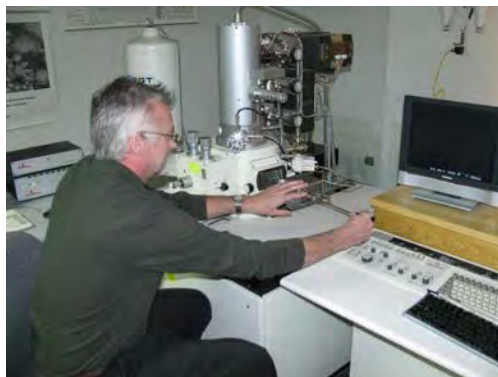
Figure 26.21 An electron microscope has the capability to image individual atoms on a material. The microscope uses vacuum technology, sophisticated detectors and state of the art image processing software. (credit: Dave Pape)
