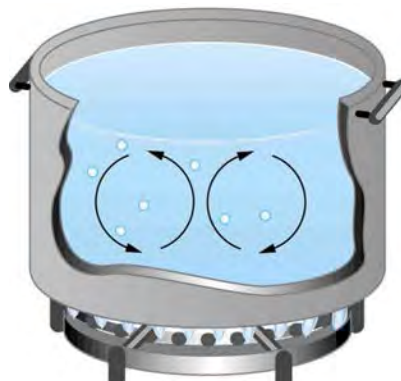
Figure 14.18 Convection plays an important role in heat transfer inside this pot of water. Once conducted to the inside, heat transfer to other parts of the pot is mostly by convection. The hotter water expands, decreases in density, and rises to transfer heat to other regions of the water, while colder water sinks to the bottom. This process keeps repeating.
