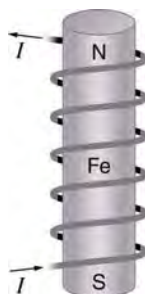
Figure 22.11 An electromagnet with a ferromagnetic core can produce very strong magnetic effects. Alignment of domains in the core produces a magnet, the poles of which are aligned with the electromagnet.
