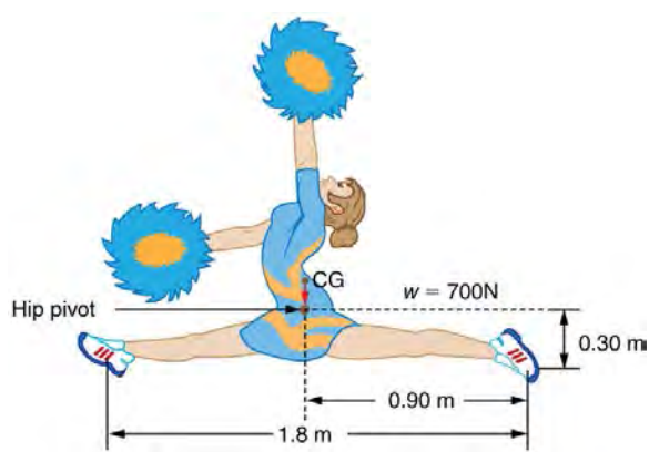
Figure 9.36 A gymnast performs full split. The center of gravity and the various distances from it are shown.
