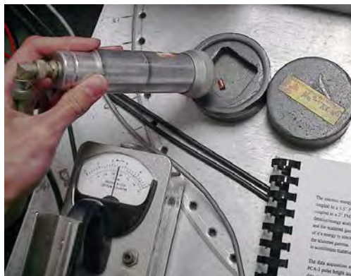
Figure 31.4 These dosimeters (literally, dose meters) are personal radiation monitors that detect the amount of radiation by the discharge of a rechargeable internal capacitor. The amount of discharge is related to the amount of ionizing radiation encountered, a measurement of dose. One dosimeter is shown in the charger. Its scale is read through an eyepiece on the top. (credit: L. Chang, Wikimedia Commons)
