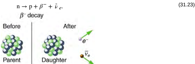
Figure 31.19 In \beta^- decay, the parent nucleus emits an electron and an antineutrino. The daughter nucleus has one more proton and one less neutron than its parent. Neutrinos interact so weakly that they are almost never directly observed, but they play a fundamental role in particle physics.
