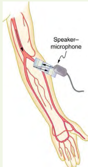
Figure 17.48 Ultrasound is partly reflected by blood cells and plasma back toward the speaker-microphone. Because the cells are moving, two Doppler shifts are produced—one for blood as a moving observer, and the other for the reflected sound coming from a moving source. The magnitude of the shift is directly proportional to blood velocity.
