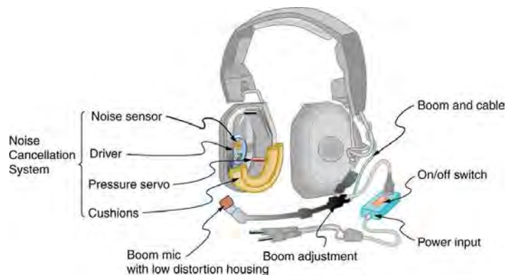
Figure 17.22 Headphones designed to cancel noise with destructive interference create a sound wave exactly opposite to the incoming sound. These headphones can be more effective than the simple passive attenuation used in most ear protection. Such headphones were used on the recording, around the world nonstop flight of the Voyager aircraft to protect the pilots’ hearing from engine noise.
