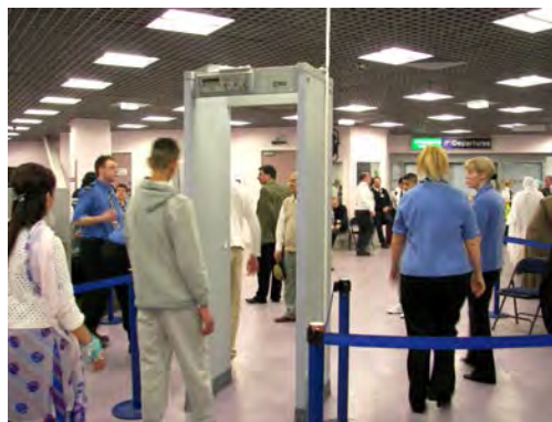
Figure 23.43 The familiar security gate at an airport can not only detect metals but also indicate their approximate height above the floor. (credit: Alexbuirds, Wikimedia Commons)
