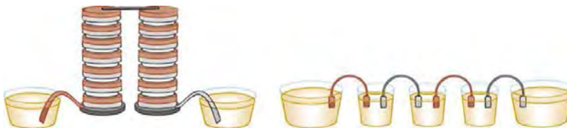
Figure 21.16 Batteries are multiple connections of individual cells, as shown in this modern rendition of an old print. Single cells, such as AA or C cells, are commonly called batteries, although this is technically incorrect.
