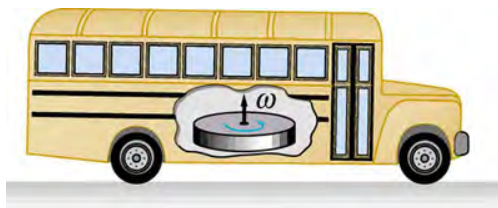
Figure 10.16 Experimental vehicles, such as this bus, have been constructed in which rotational kinetic energy is stored in a large flywheel. When the bus goes down a hill, its transmission converts its gravitational potential energy into \text{KE}_{\text{rot}} . It can also convert translational kinetic energy, when the bus stops, into \text{KE}_{\text{rot}} . The flywheel's energy can then be used to accelerate, to go up another hill, or to keep the bus from going against friction.
