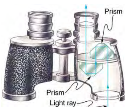
Figure 25.18 These binoculars employ corner reflectors with total internal reflection to get light to the observer's eyes.
