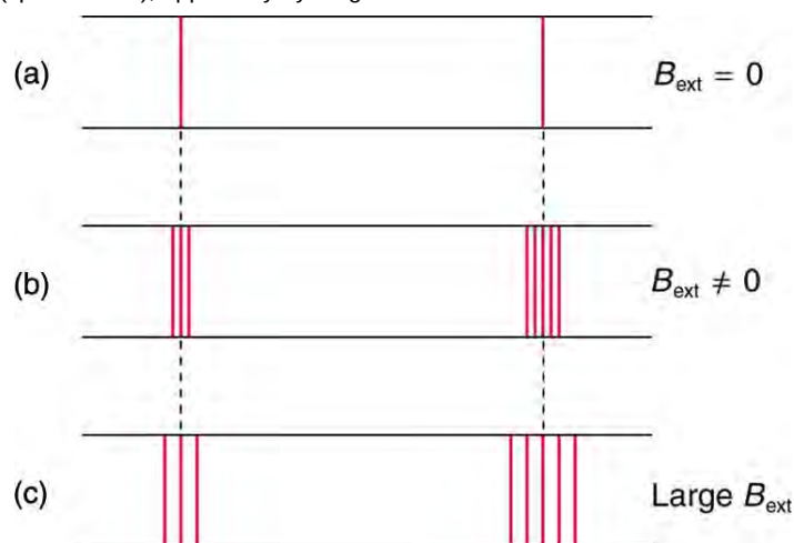
Figure 30.50 The Zeeman effect is the splitting of spectral lines when a magnetic field is applied. The number of lines formed varies, but the spread is proportional to the strength of the applied field. (a) Two spectral lines with no external magnetic field. (b) The lines split when the field is applied. (c) The splitting is greater when a stronger field is applied.
