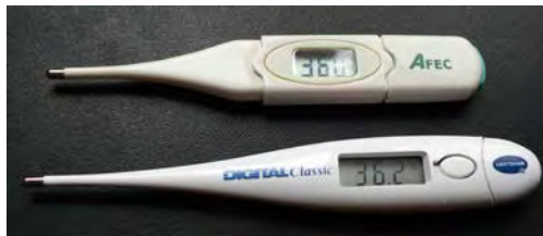
Figure 20.13 These familiar thermometers are based on the automated measurement of a thermistor's temperature-dependent resistance. (credit: Biol, Wikimedia Commons)
