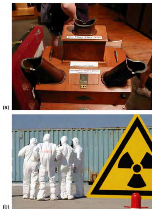
Figure 32.35 (a) This x-ray fluorescence machine is one of the thousands used in shoe stores to produce images of feet as a check on the fit of shoes. They are unshielded and remain on as long as the feet are in them, producing doses much greater than medical images. Children were fascinated with them. These machines were used in shoe stores until laws preventing such unwarranted radiation exposure were enacted in the 1950s. (credit: Andrew Kuchling ) (b) Now that we know the effects of exposure to radioactive material, safety is a priority. (credit: U.S. Navy)
