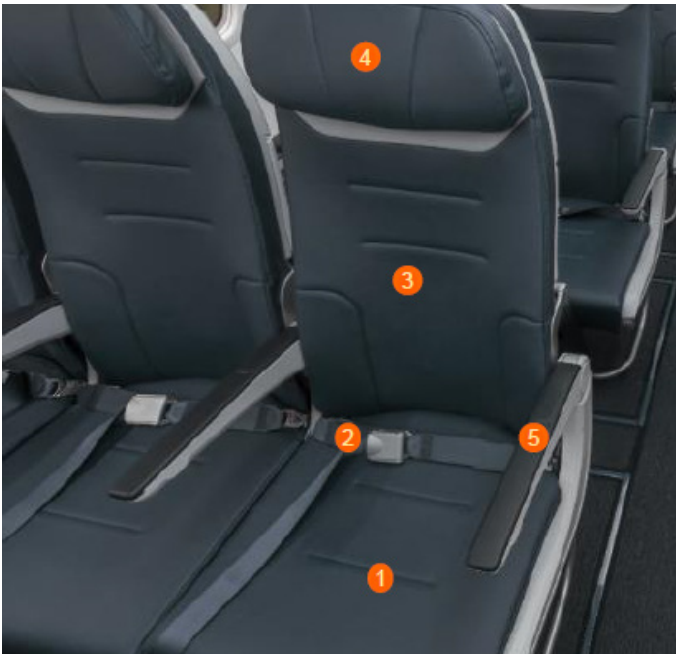
Figure 1. High-frequency touch areas of the seat are: 1) seat cushion; 2) seatbelt (buckle, latch and strap on both sides); 3) seatback cushion; 4) headrest, and 5) armrest (including seat recline button).
