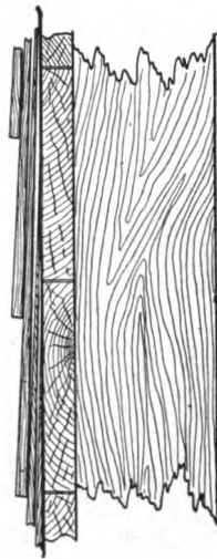
Fig. 278. Section of Shingled Wall
