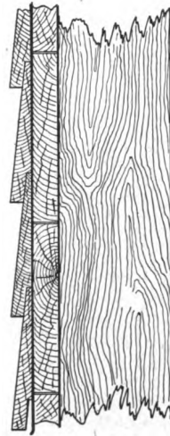
Fig. 274. Section Showing Method of Laying Siding
