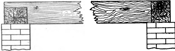
Fig. 150. Superior Floor Joist and Sill Construction
