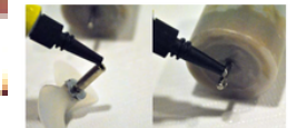
Figure 2.6-1: Adhesive on Tip of Roughened Motor Shaft and in Hollow End of Shaft Coupler
