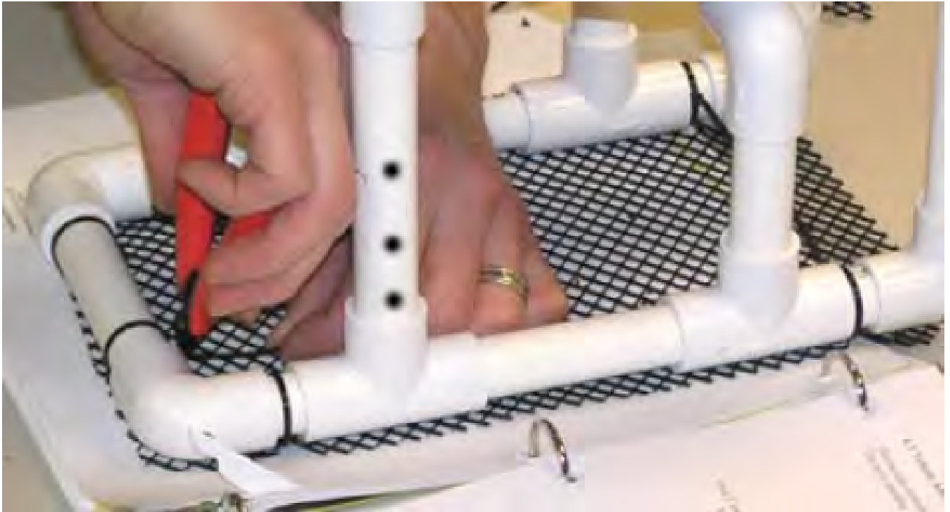
Figure 1.4-1: Payload Netting Attached to Frame
