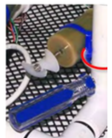
Figure 2.6-6: Thruster Angle Adjusted By Inserting a Screwdriver Through the Angle-Adjustment Holes and Tightening
