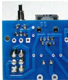
Figure 3.3-6: Bottom of a PCB Soldering All Components
