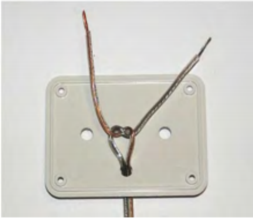
Figure 3.4-1: Power Cord Passed Through the Hole in the Box Lid, and Knotted
