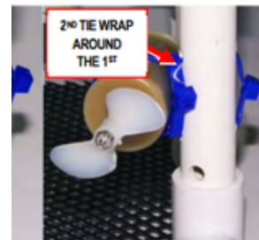
Heavy-Duty Tie Wrap Holds the Thruster in Place and a Second Tie Wrap Tightens the Thruster Tightly to the Frame
