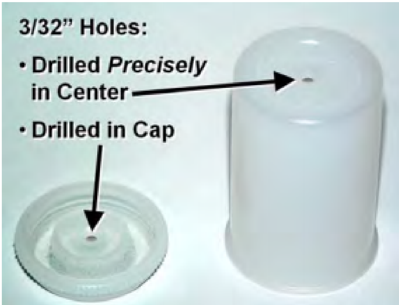
Figure 2.2-1: Holes Drilled in Thruster Housings
