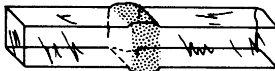
Joint "drying." Cushions harden.
