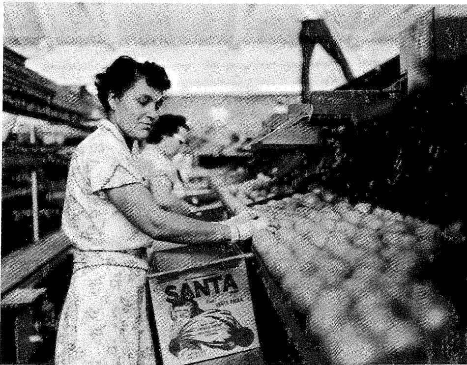
Fig. 16.2. The orange pack-out bin provides fruit at a fixed position at elbow height. All heights are adjusted so the packer can either stand or sit.
