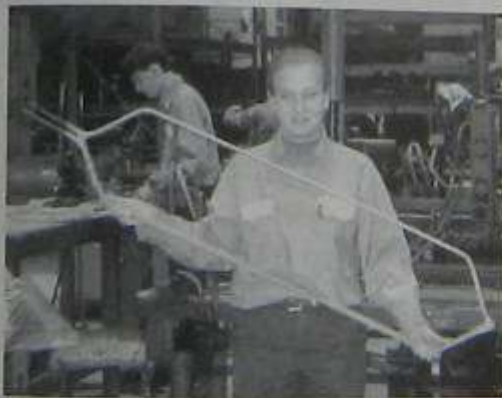
Figure 13.24b Close-up view of the preformed coil in Fig. 13.24a.
