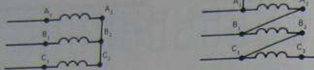
Figure 13.22f The phase may be connected in wye or in delta, and three leads are brought out to the terminal box.
