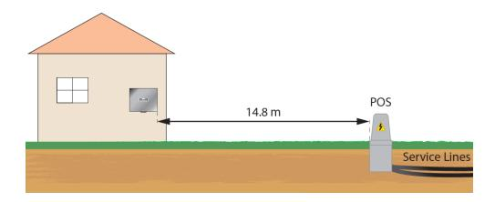
2.1.2 Select a suitable wiring system for the installation in compliance with AS/NZS 3000 Wiring Rules and local service and installation rules (SIR), and record details in the spaces provided below:
